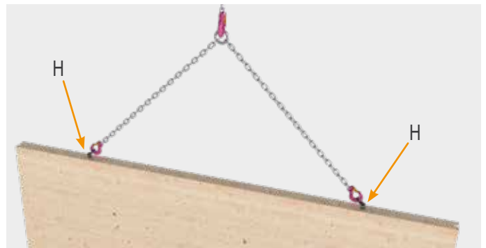
Lifting a vertical wall using two assembled Lifting Anchors Mini and ball supporting bolts (H) on the narrow side.
