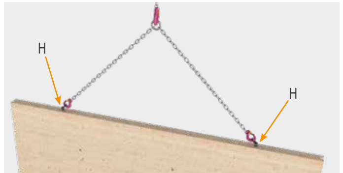
Lifting a vertical wall using two assembled Lifting Anchors and ball supporting bolts (H) on the narrow side.
