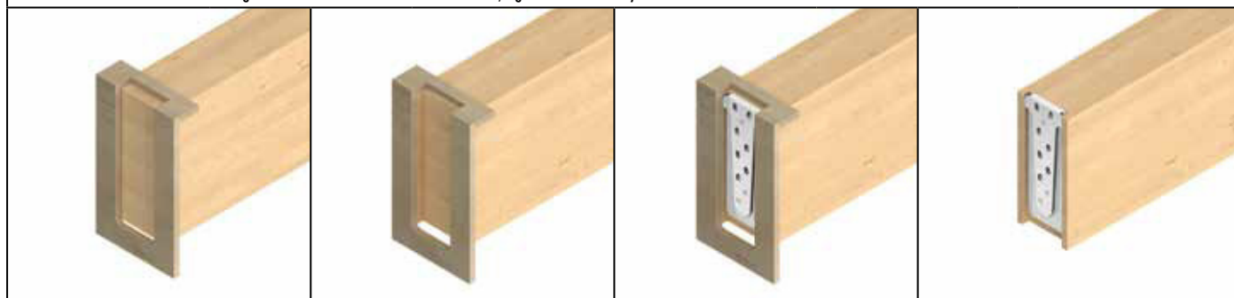
The secondary beam must be milled out at full height in the event of flush-mounted installation
