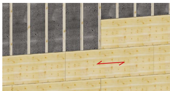
Structure verticale (mur) – pose horizontale
